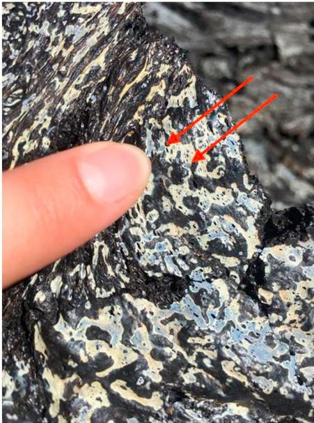
**Figure 7.** The pits created by the laser shots from the LIBS instrument are visible here (at tips of arrows). The pits are in a  $3 \times 4$  raster in the blue- and yellow-coated surface of the D1974 lava flow.
