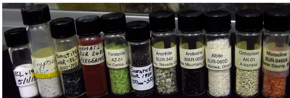
Fig. 3. Example of particulate samples used for C_p(T) measurements, available from the Arizona State University spectral library collection (Christensen et al., 2000b).
